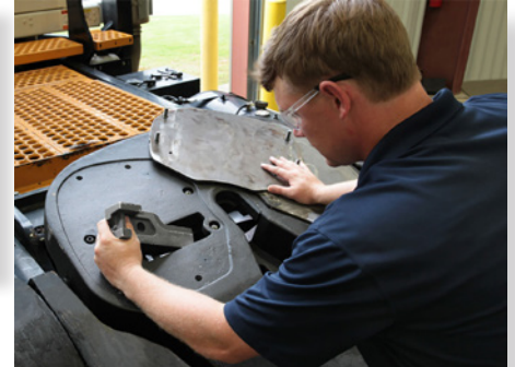
Fontaine Armor™ is easier to maintain and faster to rebuild than other terminal tractor fifth wheels. Its unique lock design enables technicians to replace critical locking components from the top side, reducing rebuild time to as little as 15 minutes instead of the up to three hours required on other yard truck fifth wheels.
