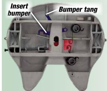
**Step 3:** Place the bumper back in position, sliding bumper tang through the operating handle guide slot and toward the tab on the side of the fifth wheel substructure.
