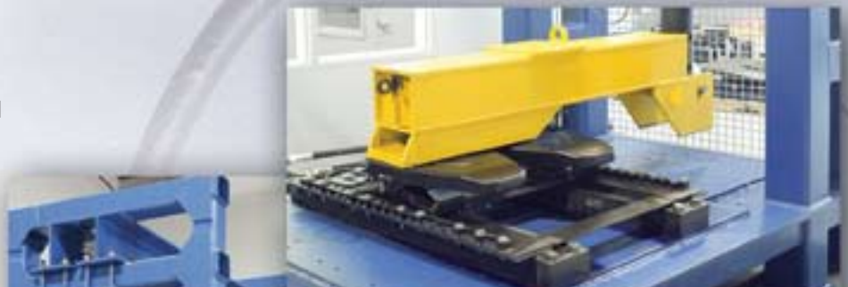
Static Load Test Frame determines vertical load rating and ultimate strength of a fifth wheel to make sure it meets EC 94/20 standards.
