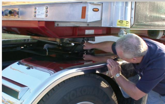
**DISENGAGE LOCK.** Pull the fifth wheel handle all the way out making sure the **handle notch** contacts the **handle retainer** that is welded to the skirt of the top plate. This will keep the handle fully extended and prevent it from retracting.
