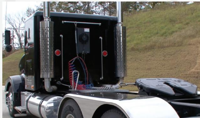
**EASE OUT FROM UNDER THE TRAILER.** Pull forward slowly until the fifth wheel clears the kingpin. Dump the air from the tractor suspension, and drive carefully away from under the trailer.
