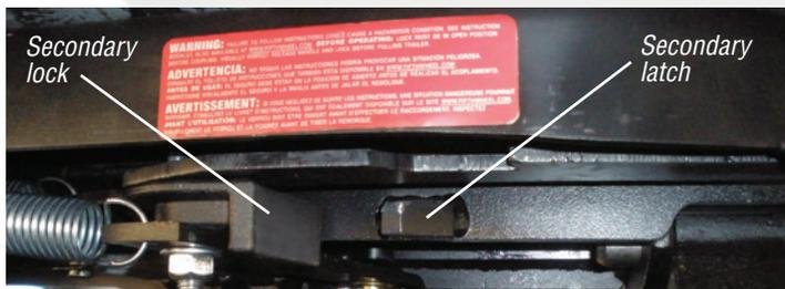
Inspect underneath the front of the top plate to verify that the **secondary lock** is properly engaged. When properly engaged, the **secondary lock** will be positioned inside the **secondary latch** toward the center of the fifth wheel (left-hand top plate shown in above photo).
