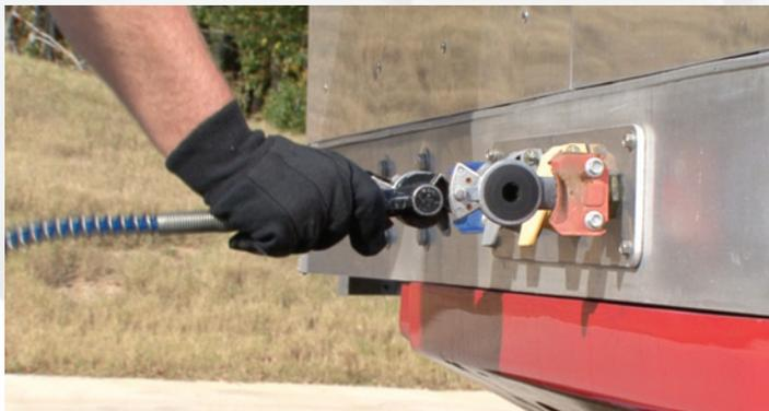
**DISCONNECT ALL CABLES.** Disconnect the air and electrical lines from the trailer.
