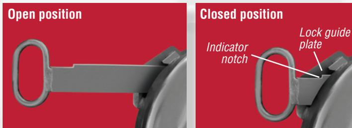
**WARNING:** If the pull handle **indicator notch** is not within the **lock guide plate** area, the lock is not properly closed and the **secondary lock** has not engaged.
