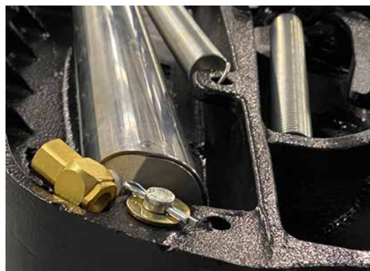
Stainless steel cylinder for in-cab air actuated models
