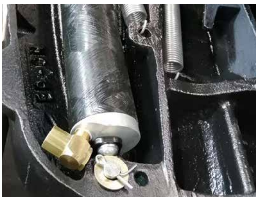
Composite cylinder for in-cab air actuated models
