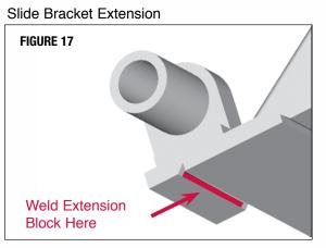
Weld Pattern For Shaft Supports
