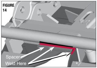
Rocker Limit Block and Guide Bar
